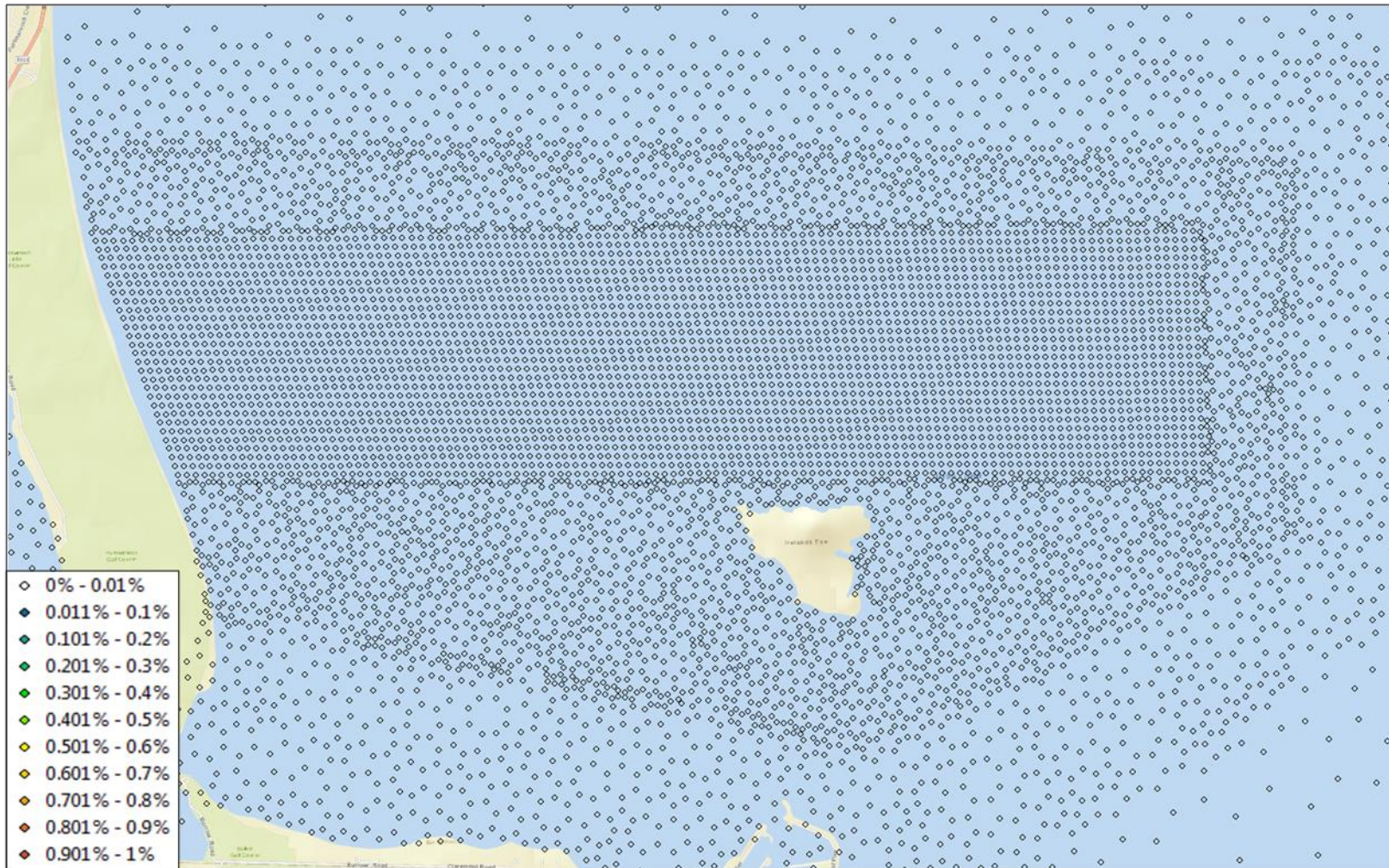
Diagram 8.6: Percentage of Time During Dredging Operation that Suspended Sediment Concentrations Exceed 100mg/l at the Water Surface
